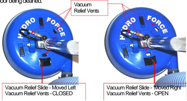
Using the SX-15 with extractors with higher air flow will generally require the vacuum relief vents to be opened more.
