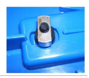
Retaining Nut aligned to secure Inner Shell
