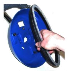
Place the Inner Shell back onto the Outer
